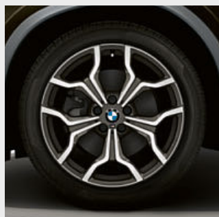
□ 19" M light alloy wheels Y-spoke 1 style 722 M, Orbit Grey, gloss-lathed with runflat tyres, wheel size 8J x 19 with 225/45 R19 tyres.
