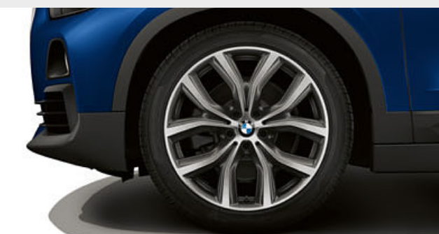
□ 19" light alloy wheels Y-spoke style 511 Orbit Grey, gloss-lathed with runflat tyres, wheel size 8J x 19 with 225/45 R19 tyres.
