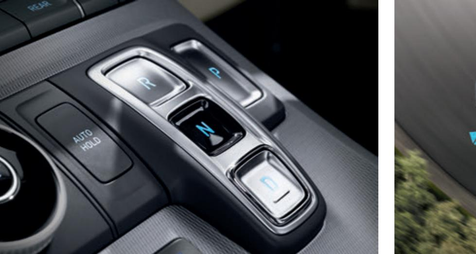
8-speed shift-by-wire automatic transmission
